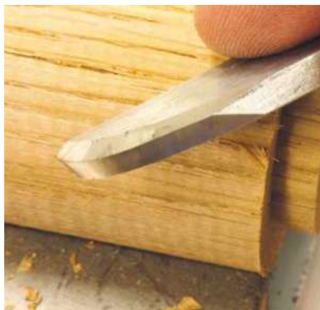
▲ Pic.11 Over the past few years Les has started to grind his scrapers like this. The bevel on the top gives it a negative rake, making the tool less likely to dig in
